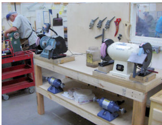
A view of the new grinding area for sharpening lathe tools.
